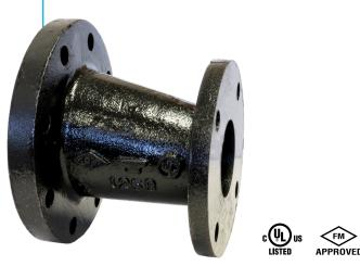
All standard or "class 125" cast iron flanged fittings are manufactured to ASME specifications and are marked 125 for pipe sizes 12 NPS (300 DN) and smaller; and have plain faces. Unless otherwise specified, cast iron flanged fittings are drilled and faced in accordance with ASME B16.1.
